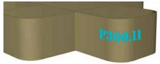
**2** Position building line (BL) as per length and width of base panel (i.e. 300:11 is 4970mm L & 3500mm W). Assemble frame with the correct cross pieces
