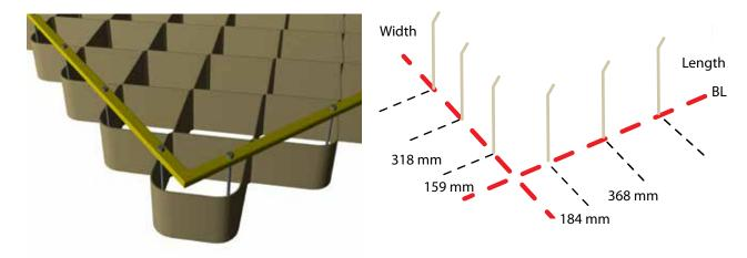
Fit the modular Profile 300 Filling Frame or insert pins at intervals of 368mm along length and 318mm along width
